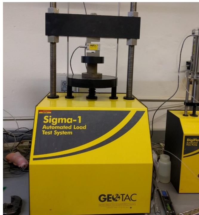
Figure C4. GeoTAC Sigma-1 Automated Load Test System
